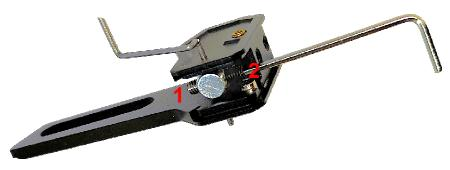
Remove the Arm wire, and replace it. Tighten the 2 side grub screw again to lock it. The Stainless Steel 1 on left in the photo must be locked strongly, the Steel Black 2 on the right just enough to stop the wire on the position wanted.
